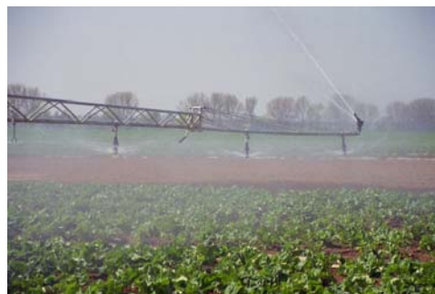
Photo 1. The water distribution manner using nozzle boom machine under windy conditions (Photo: Beinlich company)
