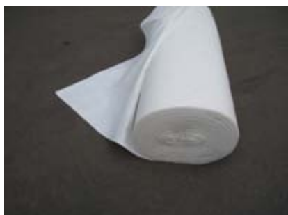
Photo 1. The geotextile material
