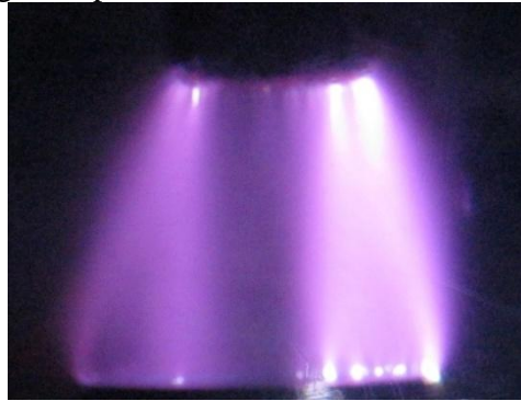
Fig. 3. Plasma of pulse electrical discharges obtained under laboratory conditions.
