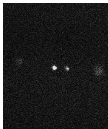
Fig. 3. Fluorescence centers of corona discharge on the conducting filament.
