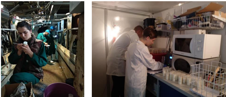
Fig. 1. CMT & collecting the milk samples for primary analysis at the farms level
