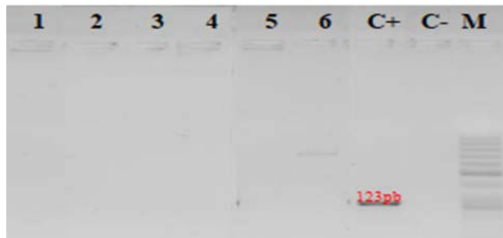
Fig. 4. PCR detection of soybean DNA by detecting lectin specific sequence. Pasteurized milk: 1, 2. Raw milk: 3, 4, 5, 6. Positive control: C+. Negative control: C-. DNA ladder, PCR marker (Thermo Scientific™ GeneRuler™ 50 bp DNA Ladder): M
