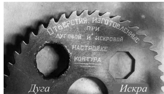
Fig. 8. Eight-sided holes made in a steel milling cutter by arc and spark electric discharges.
