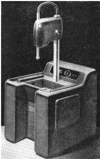
Fig. 40. Physical configuration of an electrospark installation of the W/SM type (Wickman-Erodomatic).
