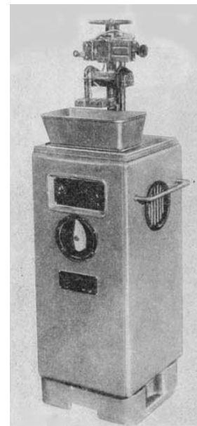
Fig. 32. LKZ-57 installation for production of fine blanking dies, profiled dies, and drawing dies.
