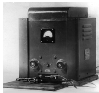
Fig. 25. Electrospark installation for alloying metal surfaces of the Kharkov tractor plant.
