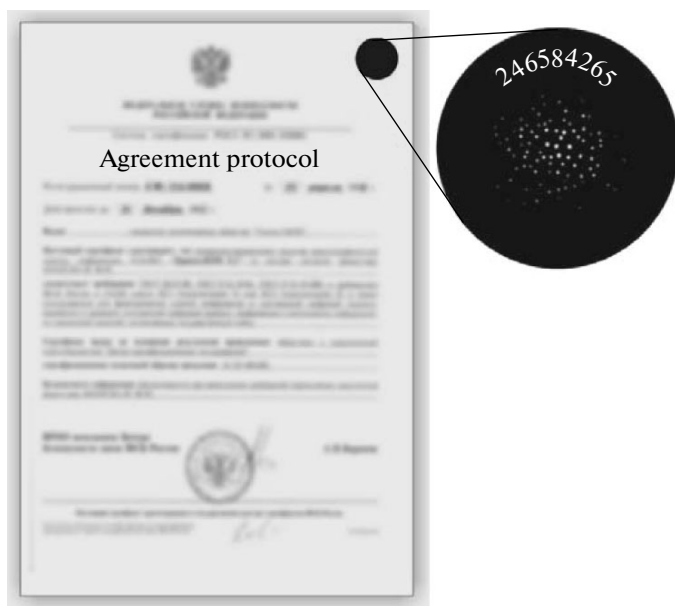
Fig. 2. A high-security document protected using an individual numeric code using electric-discharge technology.
