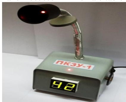
Fig. 1. The appearance of the electronic device PKUZ-1, which diagnoses the functionality of the visual analyzer and motor fatigue of tennis players
