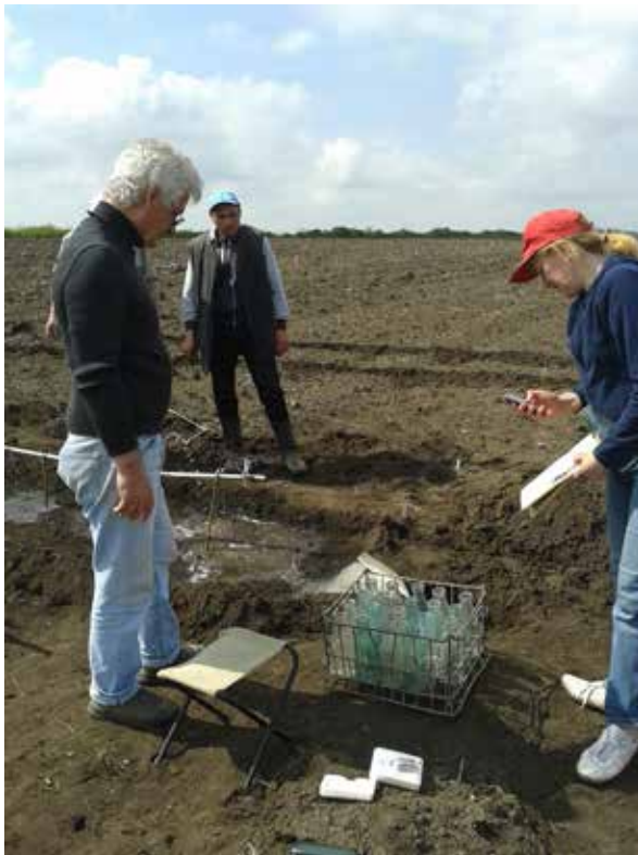
Fig. 3 and 4. Determining the volume and turbidity leaks under the influence of artificial rain of certain intensity
