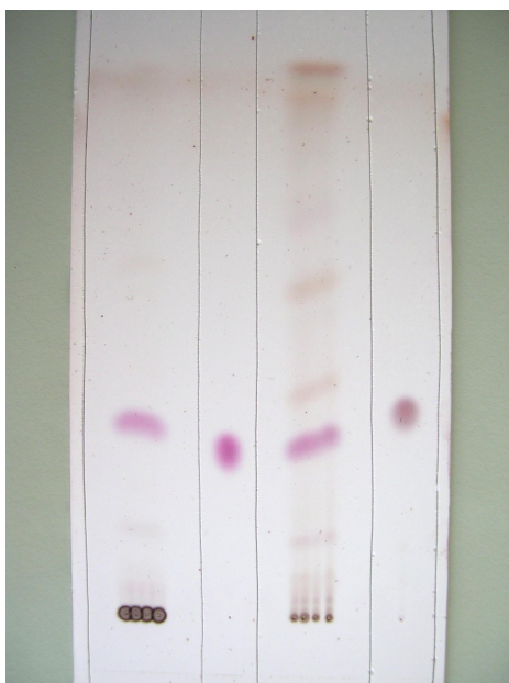
Fig. 6. TLC analysis of methanolic and dichloromethane extracts of Prunellae herba (1 - MeOH extr.; 2 - ursolic acid; 3- \text{CH}_2\text{Cl}_2 extr.; 4-oleanolic acid)
