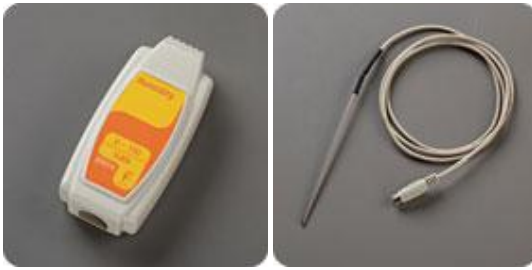
Fig. 3: Humidity and Temperature sensors provided with Nova5000 bundle.
