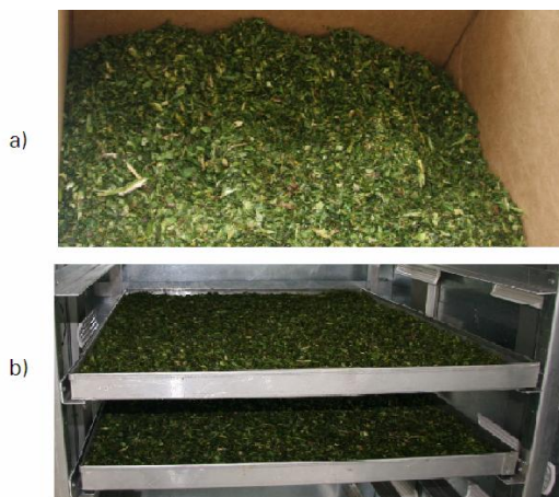
Fig.2. Minced celery: a) material sample; b) distributed in drawers, ready to dry.
