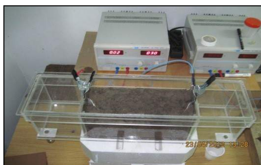
Fig. 1 - Experimental installation of electro-flushing (top view)
