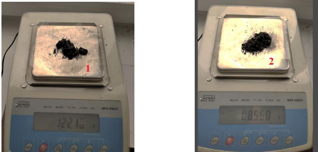
1—with the influence of the magnetic field, 2— without the influence of the magnetic field
