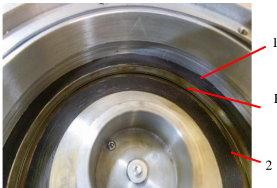
1 – surface of the pole attachment, 2 – surface of the tooth on the FF seal shaft.
