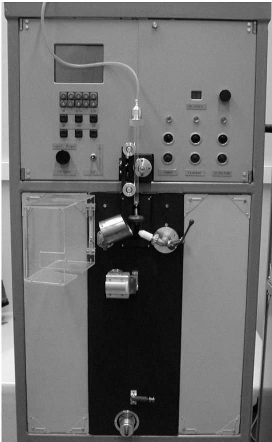
Fig. 1a. Machine for the preparation of CGCFMWs by the Ulitovsky–Taylor method (produced at AMOTEC Ltd, Moldova).
