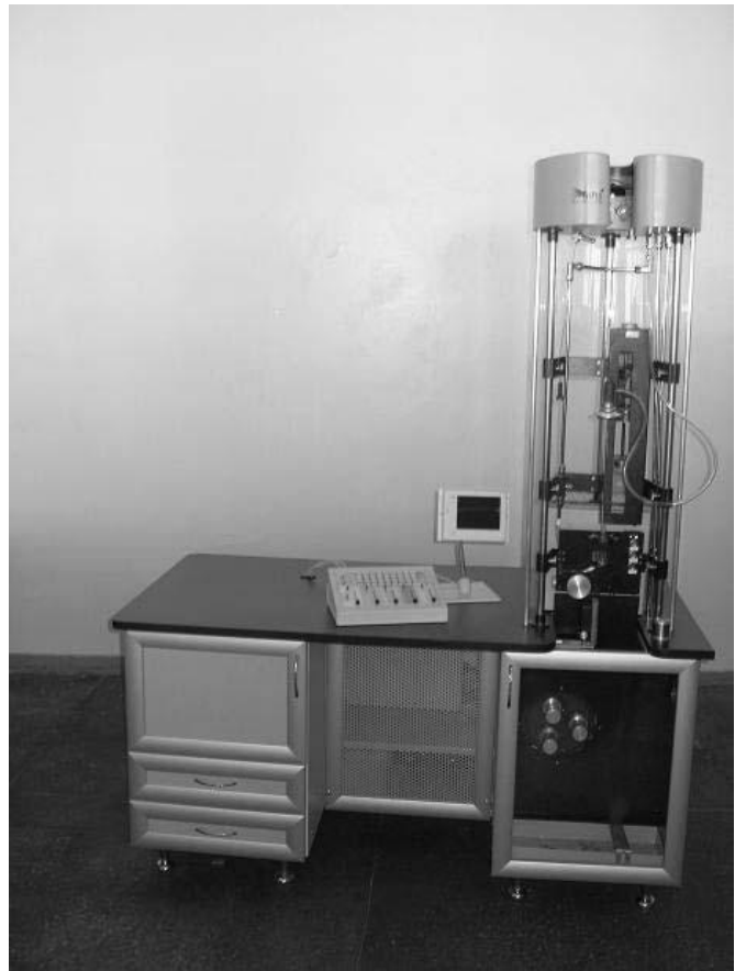
Fig. 1b. Novel machine for the preparation of CGCFMWs by the Ulitovsky–Taylor method (produced at MFTI Ltd, Moldova).
