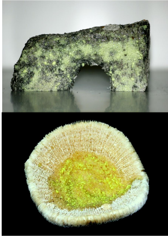
Fig. 2. Artificial block from concrete and sand covered by \text{SrAl}_2\text{O}_4:\text{Eu}^{2+}, \text{Dy}^{3+} (top) and real coral with phosphor inside (bottom)
