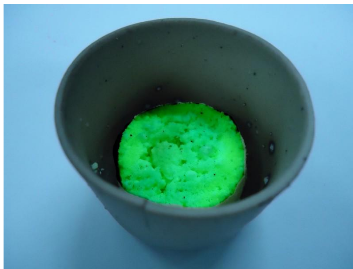
Fig. 1. Bright luminescence of \text{SrAl}_2\text{O}_4:\text{Eu}^{2+}, \text{Dy}^{3+} based phosphor in the open air under sun light excitation.
