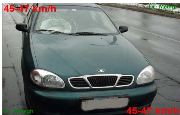
Figure 2. Impact at speeds of approx. 45-60 km/h.
