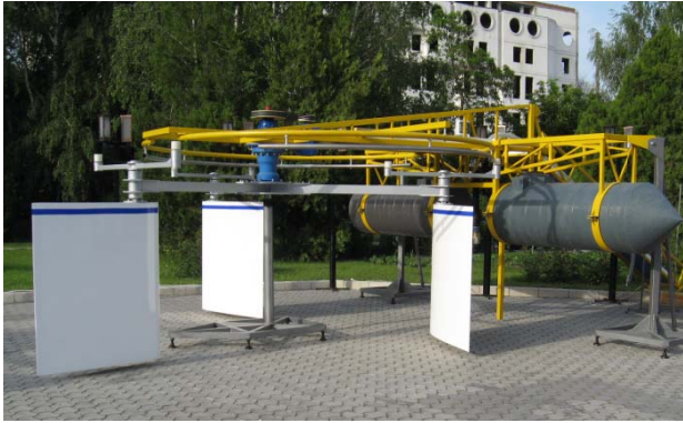
Figure 1. Micro-hydro power station with 3 hydrodynamic blades.
