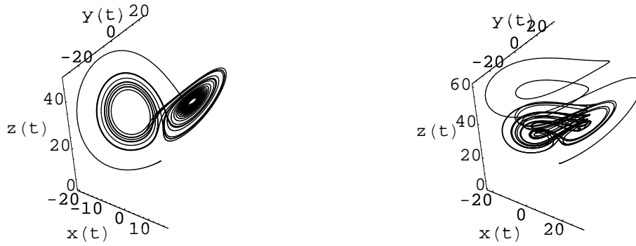
Figure 1. a) The orbit of the Lorenz system for a = 10 , b = 8/3 , c = 28 and the initial condition (-0.04, -0.3, 0.52) (left); b) The orbit of the Chen system for a = 35 , b = 3 , c = 28 and the initial condition (-0.1, 0.1, 0.4) (right)
