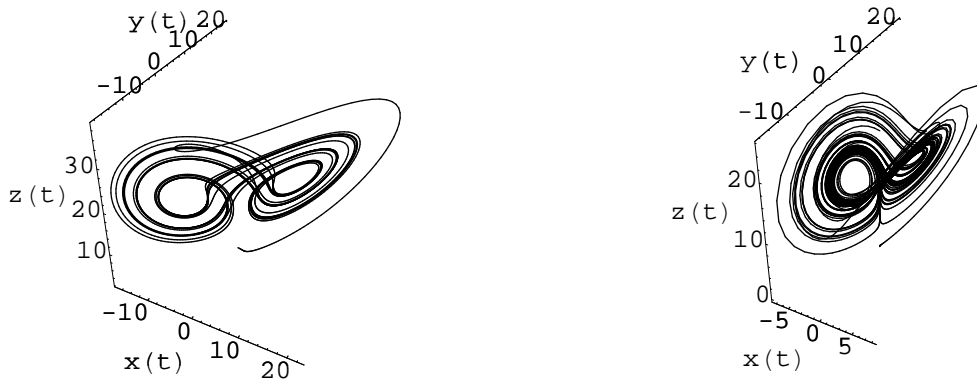
Figure 2. a) The orbit of the Lü system for a = 36 , b = 3 , c = 19 and the initial condition (-1, 0.1, 4) (left) ; b) The orbit of the T system for (a, b, c) = (2.1, 0.6, 30) and the initial condition (0.1, -0.3, 0.2) (right)
