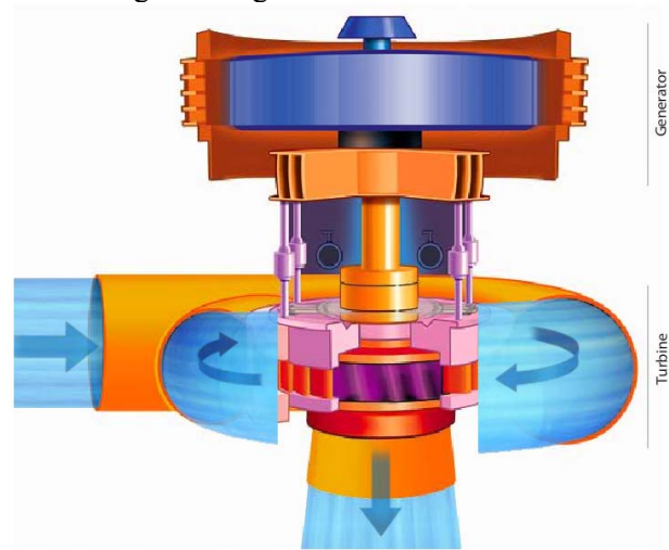
Figure 1. Cross-section view of a generating unit, update 10.04.13[1].
