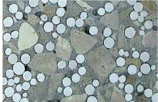
Figure 3. Typical distribution of macrofiller particles between coarse aggregate grains.
