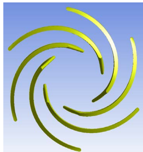
Figure 4. Geometry of the pump impeller blades obtained in ANSYS DM.
