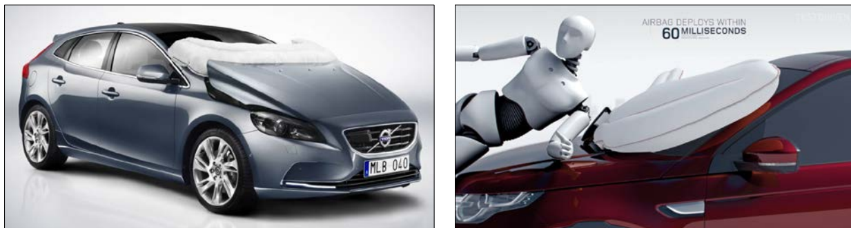
Figure 4. Pedestrian Airbag System, PAS [5, 25].
