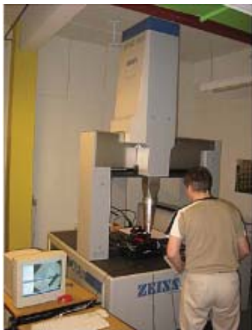
Figura 2.7 Left: Reference measurements with a high-end coordinate measurement machine (accuracy 3 microns). Right: Scan of an implant bar reference object with errors in the insertion direction [in microns]
