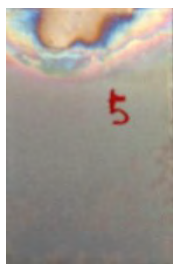
Fig. 10a. The surface morphology of MAO coating after treatment 5 s (NaOH: 0.02 mol/L).
