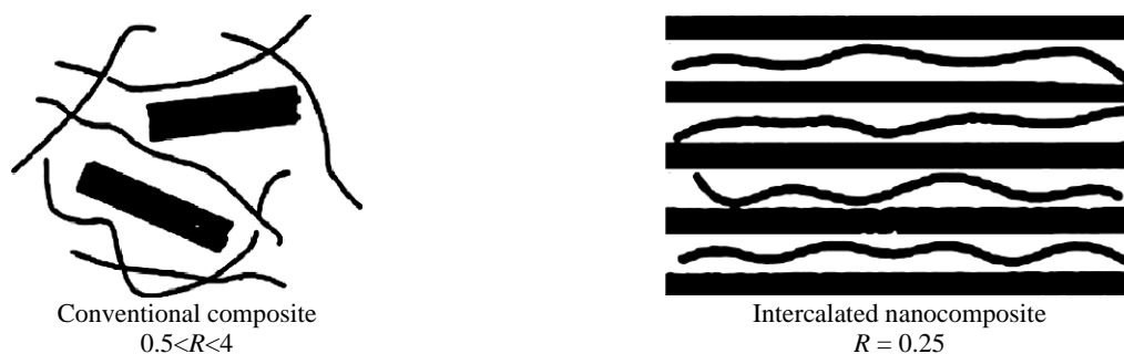
Fig. 5. Main types of intercalated nanocomposite.
