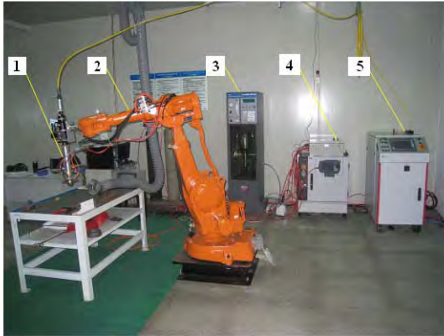
Fig. 2. The general view of industrial robotized system based on diode laser Coaxial with powder nozzle laser beam focusing system; 2 –Robot; 3–Feeder; 4–Robot controller; 5 – Fiber-Coupled Diode Laser
