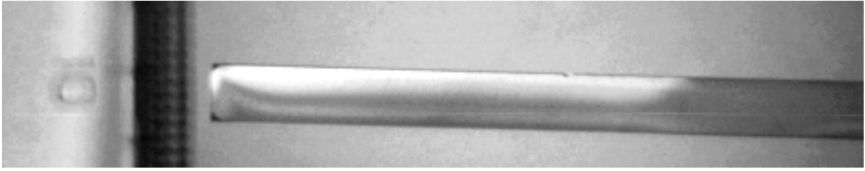
Fig. 6. Picture of remaining tensions on the butt end of rectangular plate from the optical glass after electronic treatment of its surface through a mask with next cooling after a chart (fig. 2)
