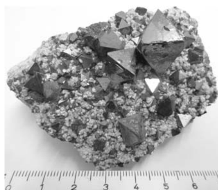
Figure 3. Geological octahedrally shaped magnetite crystallised on feldspar and quartz found in Bolivia (photo by S. Malik).
