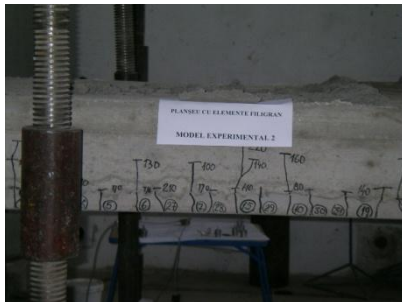
Figure 8. Experimental model in failure stage
