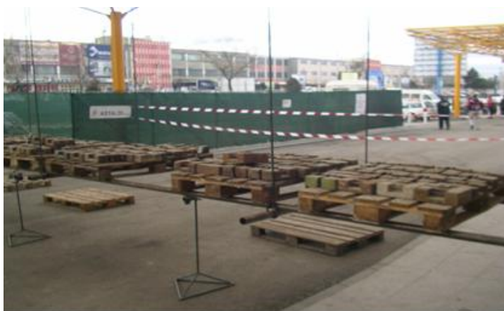
Fig. 3. Loading at the maximum reference level of the test load.
