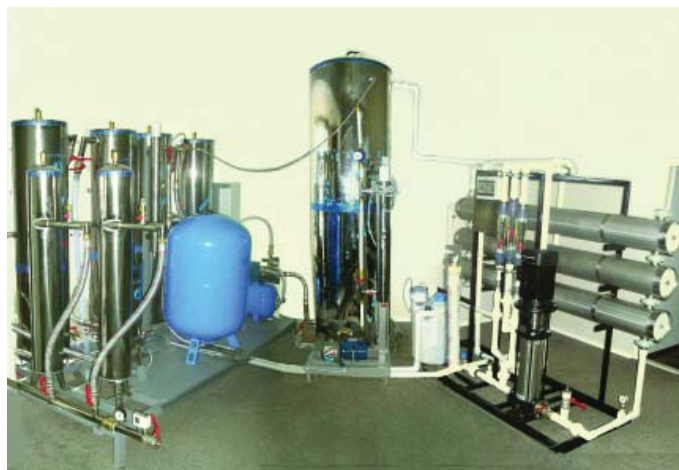
Fig.3. Multifunctional module installation “Vega-3UM” with productivity of 5000 liters per hour
