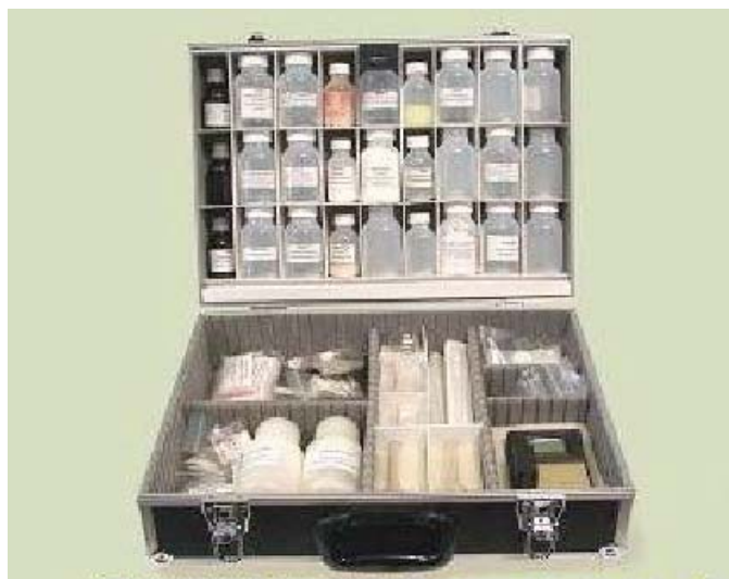
Fig. 4. Portable laboratory "Aqua-test" for monitoring water quality.
