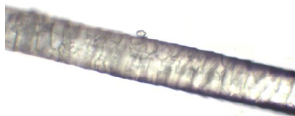
Fig.4. Microscopic image of washed wool fiber (30% lye/ 20x magnification degree)
