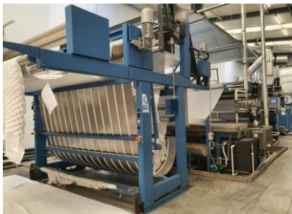
Fig. 1: Equipment for the treatment of textile materials - Squeezing Pader Machine
