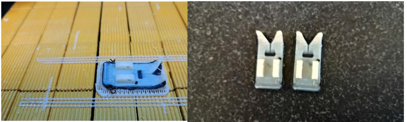
Fig. 4: The redesigned product manufactured with Inspire 200 3D printing
