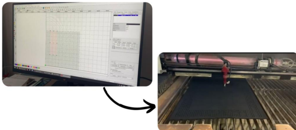
Fig. 4: The process of laser cutting the felt for the canva.
