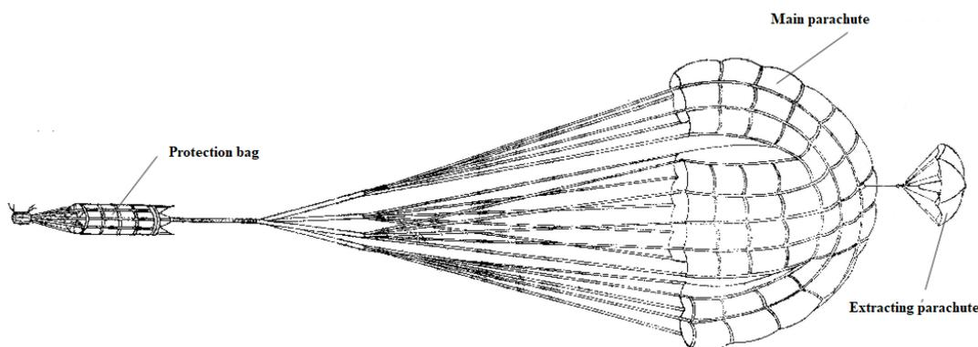
*Fig. 2: Diagram of the braking parachute assembly*
