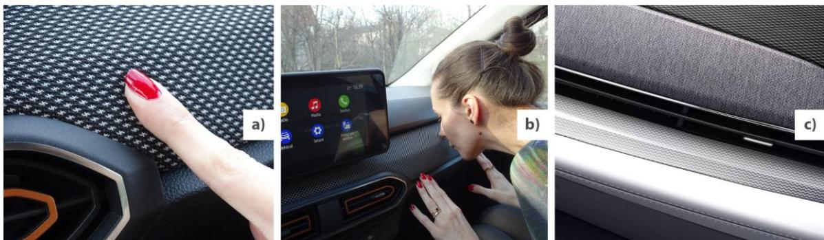
**Fig. 2:** a) Padded textile insertion (Dacia Sandero Stepway 3); b) Simulation frontal accident -the padded area ensures frontal protection to passengers; c) Padded textile insertion applied on the dashboard of Ford Mustang Mach – E 2021 vehicles
