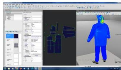
**Fig. 5:** Simulation of PPE system for intervention in emergency situations that integrates the inner layer (in contact with the skin) - Underwear PPE, intermediate layer (base) – Duty uniform and specialized PPE for interventions in extreme weather conditions
