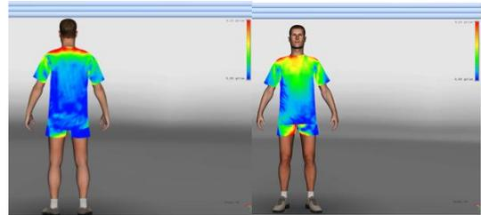
**Fig. 2:** Inner layer simulation – Underwear PPE: Suit consisting of a short-sleeved blouse and shorts
