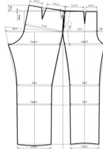
Figure 1: Basic pattern developed according to the MUPI CAER method
