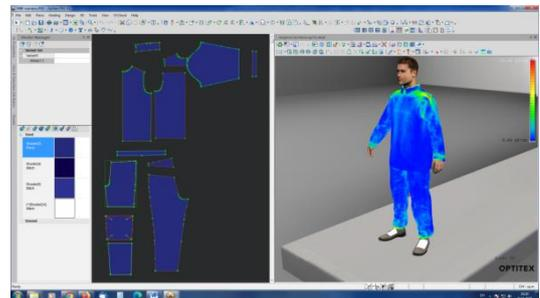
**Fig.3:** Simulation of the PPE system for intervention in emergency situations that integrates the inner layer (in contact with the skin) - Underwear PPE and the intermediate layer (base) – Duty uniform
