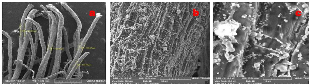
Fig. 5: SEM micrographs of treated immature coconut fibers
