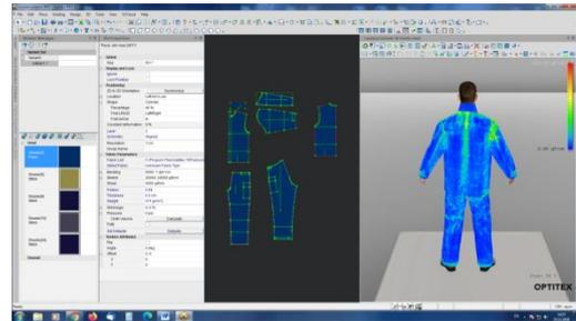
**Fig.4:** Simulation of PPE system for intervention in emergency situations that integrates the inner layer (in contact with the skin) - Underwear PPE, intermediate layer (base) – Duty uniform and specialized PPE for firefighters
