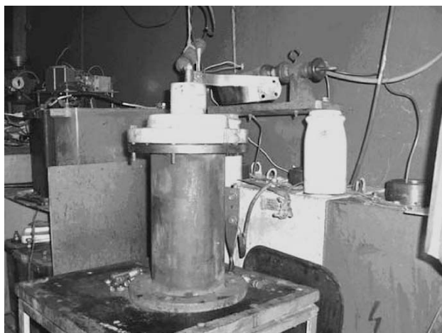
Fig. 1. Electric-discharge installation and reactor for nanocarbon synthesis.
