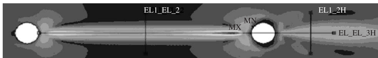
Fig. 2. Through-flow rate contour diagram in the presence of “long” bipolar jets beyond the bounds of the passive electrode.
