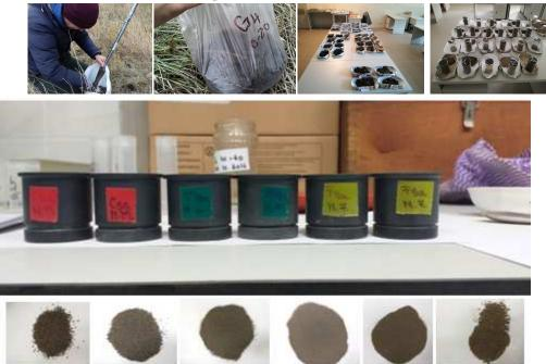
Figure 3. Soil sampling, preparation of samples for transport and storage, respectively making determinations regarding the classes of aggregates resulted from sieving soil samples
