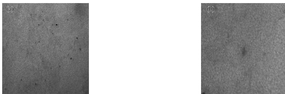
Fig. 2. Optical microscopy images of DCM solvent bonding of polycarbonate at (a) 10X and (b) 5X magnification.
