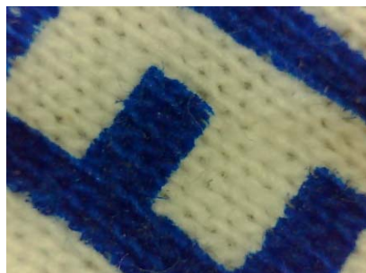
Fig. 7. Microscopic appearance of the knit printed surface by using screen printing process, z = 200x .
