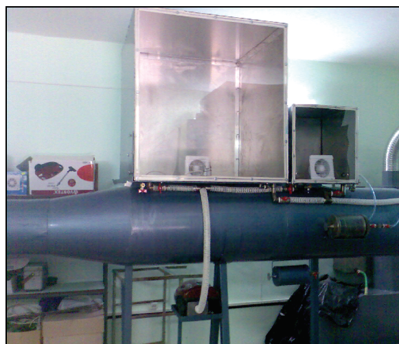
Fig. 2. A fragment of the HAT with a system for sampling and dilution of aerosol.
