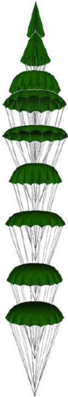
Figure 3. 2m Flat Circular Parachute Inflation Time Lapse Images
