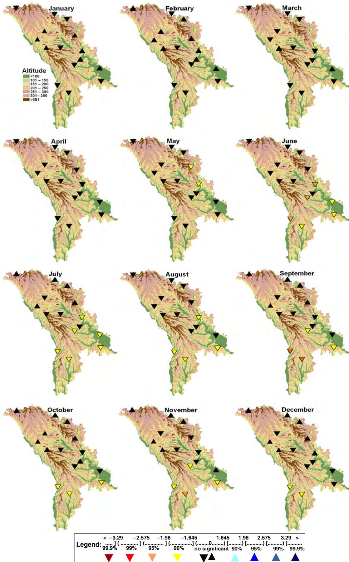
Figure 5. Spatial distribution of 6-month SPEI trend based on Mann–Kendall Z statistic at 15 stations in the RM.
