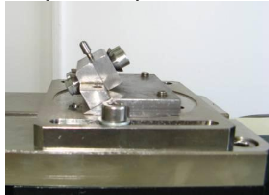
Fig.4: Clamping and positioning device
