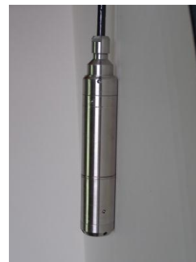
Fig. 1. Physical configuration of the TPH-485-0,06 transducer.
