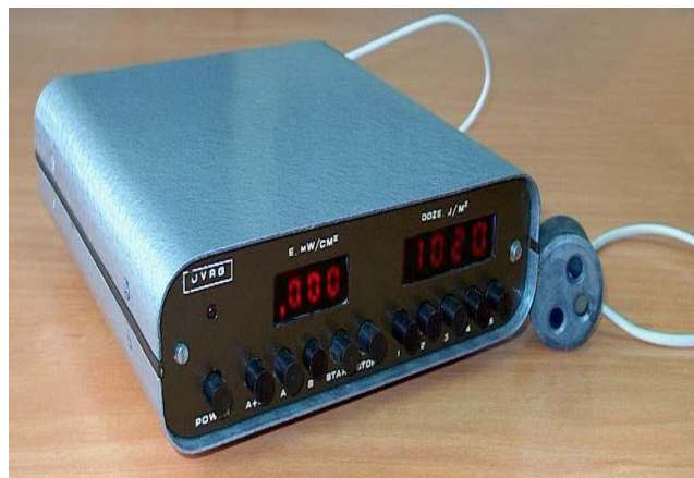
Fig. 4. The measurement device with the digit display of UV radiation with the intensity in limits of values 10^{-4} ÷ 2 \cdot 10 mW/m 2 the spectral domains, nm: 280÷400, 320÷400, 320÷360; the dose - 0 ÷ 1.6 \cdot 10^5 J/m 2 .
