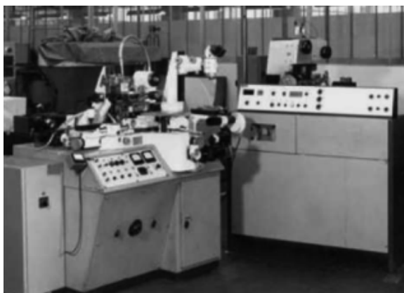
Fig. 21. Electrosark coordinate installations: (at the right) A207.23 and (at the left) A207.27 with an embedded thyatron pulse generator with an Olivetti NC system at the company.
