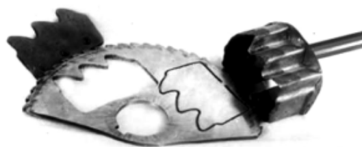
Fig. 7. Carving of a saw element by trepanning.
