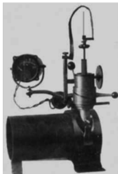
Fig. 3. Device for removing broken instruments from the shells of Katyusha projectiles (the early 1940s).
