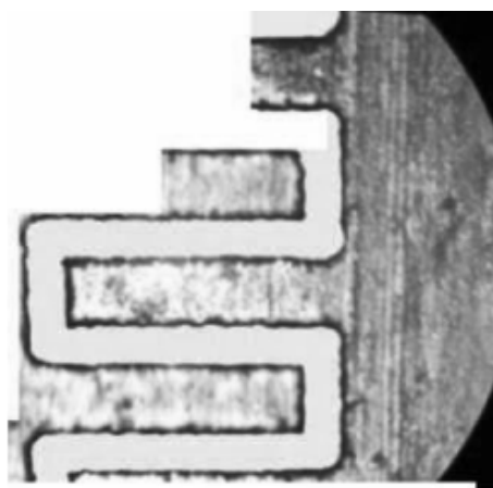
Fig. 29. Portion of an SWS BWT produced using a 15- \mu\text{m} electrode wire. A groove of 18^{+2}_{-2} \mu\text{m} ; the pins have a width of 36^{-2} \mu\text{m} and a height of 0.16 mm.
