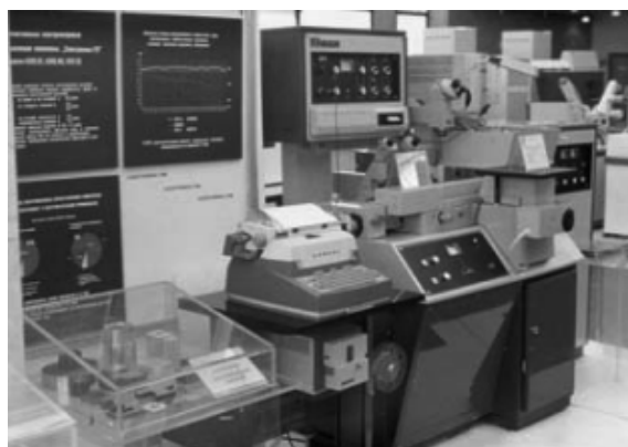
Fig. 17. Electrospark coordinate installation based on A207.23 with a thyatron pulse generator and an NC system at the exhibition of electronic engineering in Moscow.
