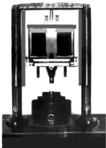
Fig. 4. First electrospark installation with a vibrator (1944).
