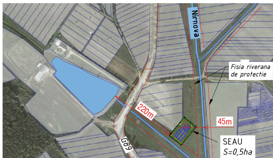
Figure 3.6. Framing of WWTP with biological filters for Cluster 1
