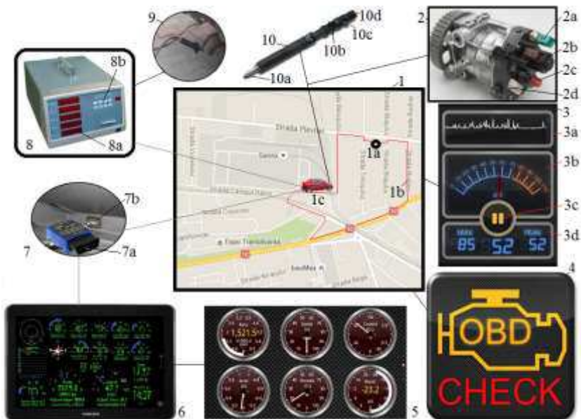
Fig. 1. Setting the protocol for communication, transfer and displaying available data from ECU. 1-Test track configuration, 1a-Start/stop location, 1b-Track sector, 1c-Tested vehicle, 2- Injection pump, 2a-Temperature sensor, 2b-Fuel flow actuator, 2c-High pressure output, 2d-Injection unit, 3-Digital phonometer, 3a-Graphic display, 3b-Analogic display, 3c-Digital operation key, 3d-Digital display, 4-Digital label, 5-Analogic interface, 6-Electronic device, 7-OBD connection, 7a-OBD interface, 7b-OBD socket inside vehicle., 8-Portable gas analyzer, 8a-Digital display, 8b-Operation panel, 9-aquisition terminal, 10-Delphi injector, 10a-Nozzle, 10b-Electric connection, 10c-Injector return, 10d-high pressure connection.
