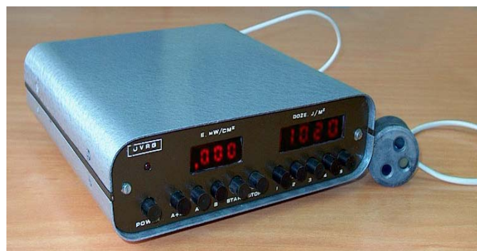
Figure 5. The measurement device with the digit display of UV radiation with the intensity in limits of values 10^{-4} ÷ 2 \cdot 10 mW/m 2 the spectral domains, nm: 280÷400, 320÷400, 320÷360; the dose - 0 ÷ 1.6 \cdot 10^5 J/m 2 . The current supplying – 220 V
