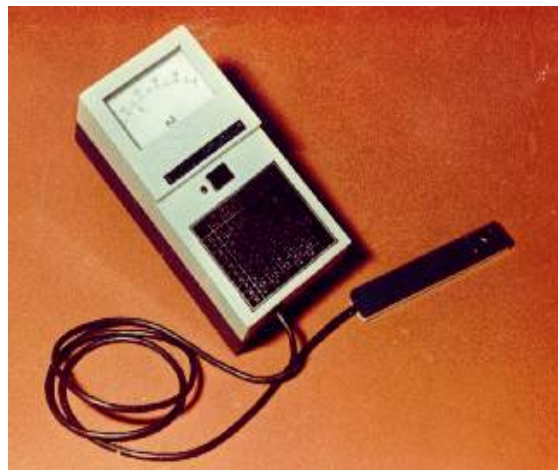
Figure 4. The device with logarithmical scale for the measurement of intensity values in the limits of 10^{-4} ÷ 10 mW/cm 2 from the range of wavelengths 280÷400 nm. The supplying is 4.5 V
