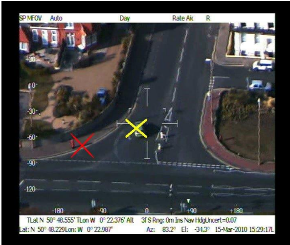
Figure 6. Kalman filter (Red) and OT-MACH filter tracker (Yellow)
