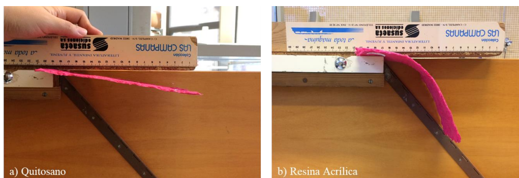
Fig. 4: Flexural rigidity comparison by binder
