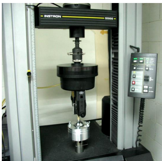
Fig. 2: A photograph of the fabric bagging tester.
