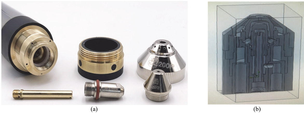
Fig. 2. Solidworks design of hydrogen plasma torches with nozzle diameter 1.5 and 2.5 mm (a) Industrial plasma torch; (b) 3D drawing of redesigned hydrogen plasma
